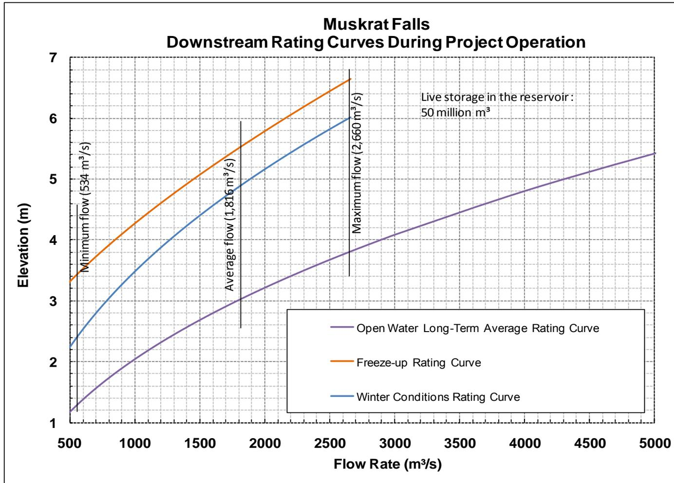
Figure 2-1: Downstream Rating Curves
