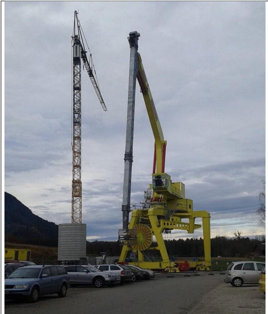
Photo 1: Trash Rack Cleaning System erected at Muhr's fabrication facility yard
