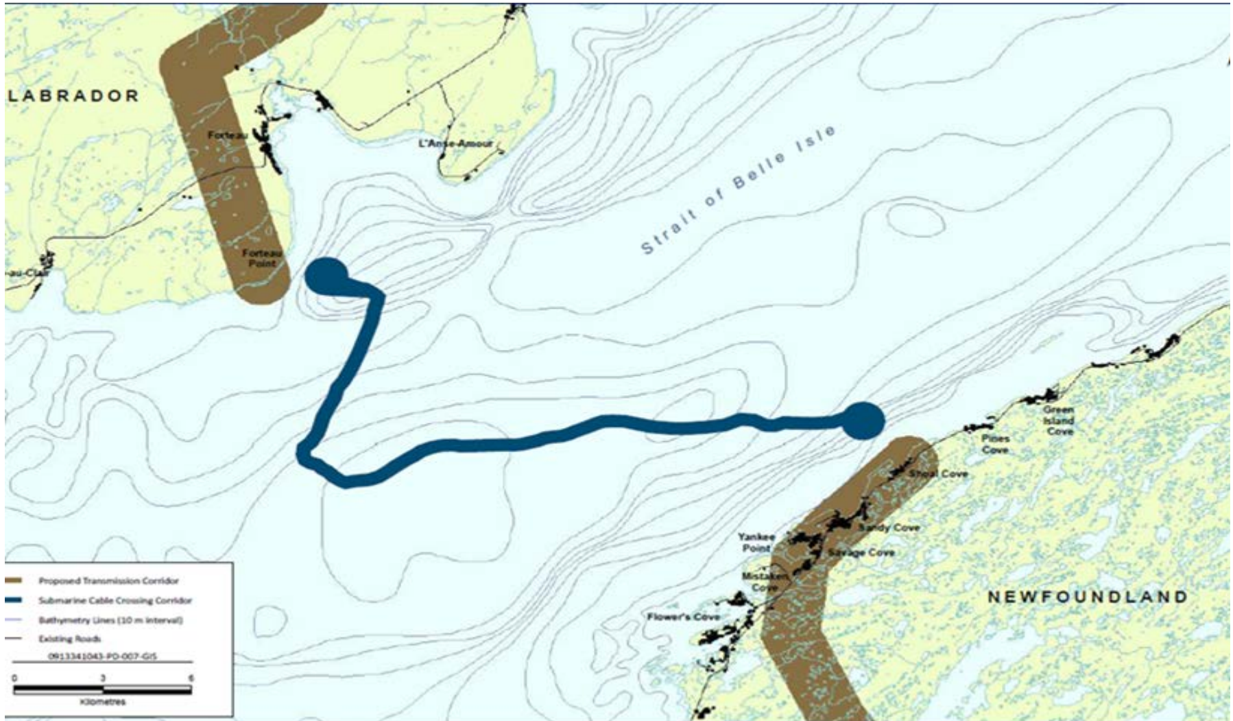
Figure 4-1 - Strait of Belle Isle Submarine Cable Crossing
